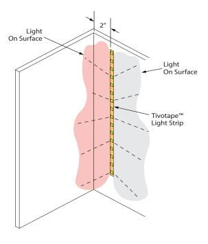
**Note 2:** In applications where multiple strips of Tivotape<sup>™</sup> are reflecting on a common surface, it is recommended that the tape be mounted at least 2″ away from the reflecting surface and oriented with the same edge of Tivotape<sup>™</sup> mounted closest to the outside edge, as shown. Note the position of the lead end.
